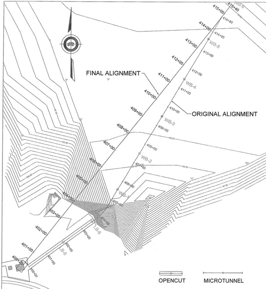
**Figure 6, Final Design – Plan View**
