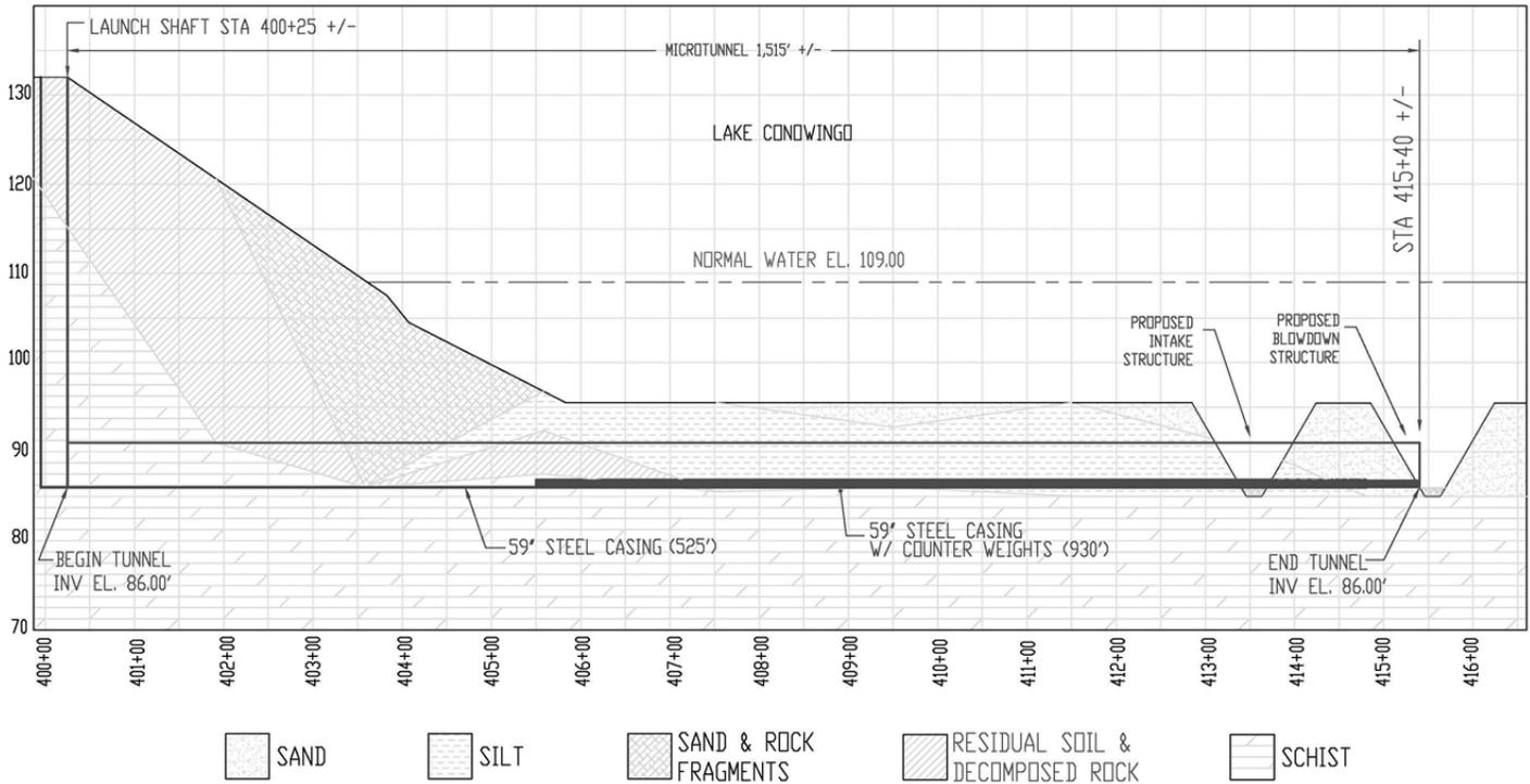
**Figure 5, Final Design – Profile View**
